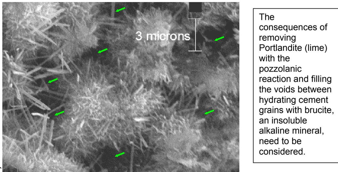
**Figure 1. Partially hydrated Portland cement paste (after Soroos, 1999<sup>4</sup>).**
