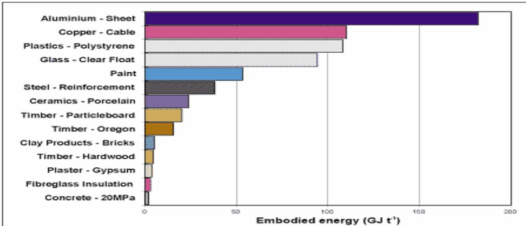
Figure 10 - Embodied Energy of Building Materials<sup>48</sup>
