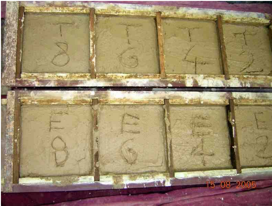
Figure 4 - Lance Collins Testing Cast Mud Bricks.
