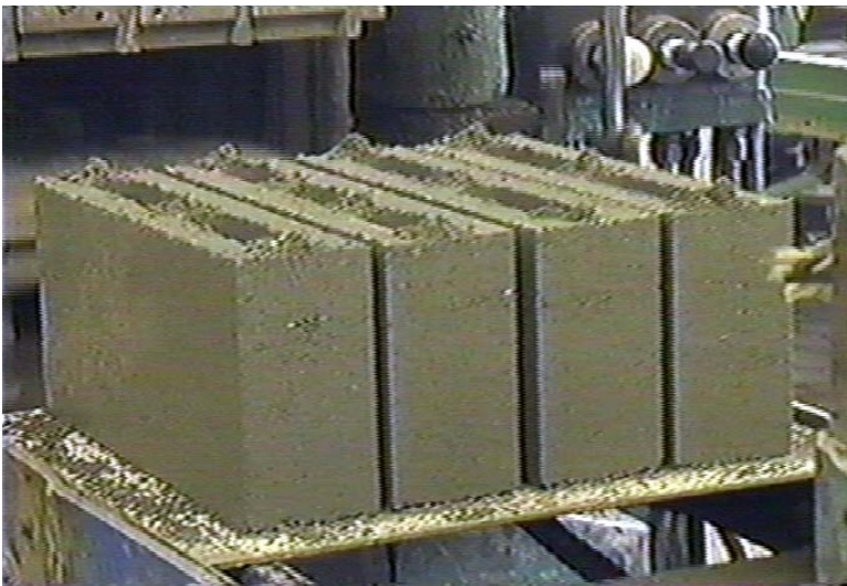
Figure 2 - Eco-Cements Coming out of a Block Machine
