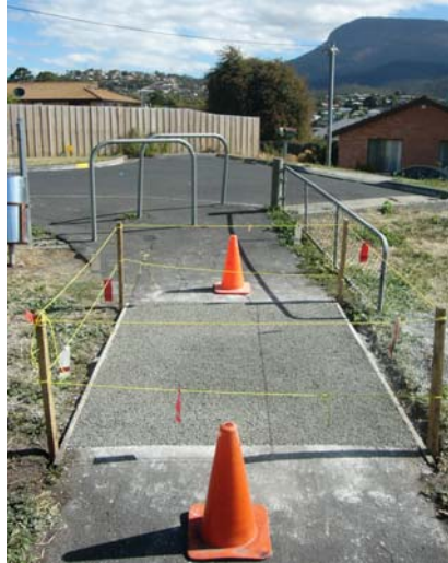
Figure 5 - A Porous pavement Experiment in Tasmania
