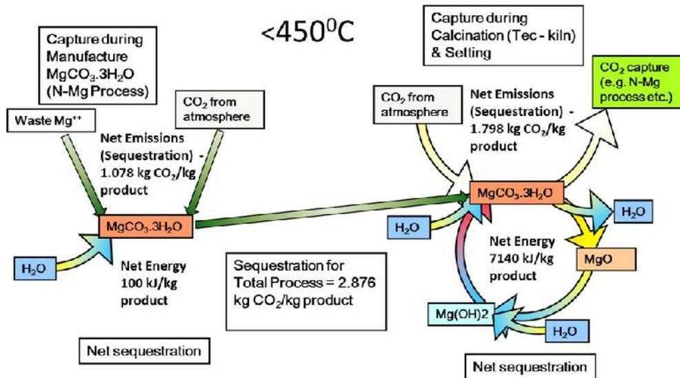
**Figure 6 – Sequestration capturing CO<sub>2</sub> from the air in the N-Mg process using TecEco’s Tec-Kiln**
