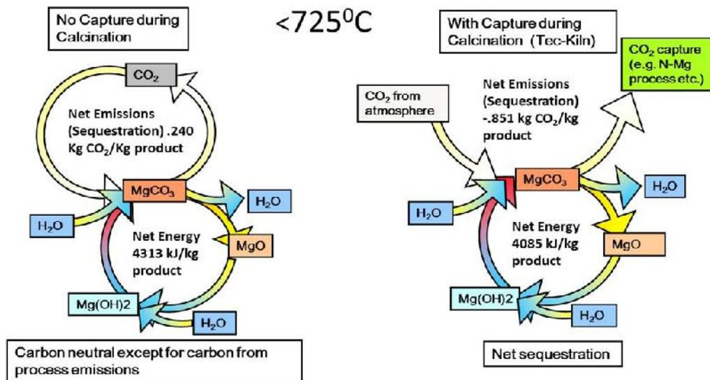
Figure 4 – Manufacture of MgO from Magnesite with and without Capture
