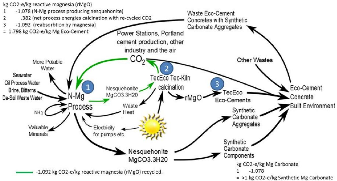
**Figure 5 - The N-Mg Sub-Process of Gaia Engineering**
