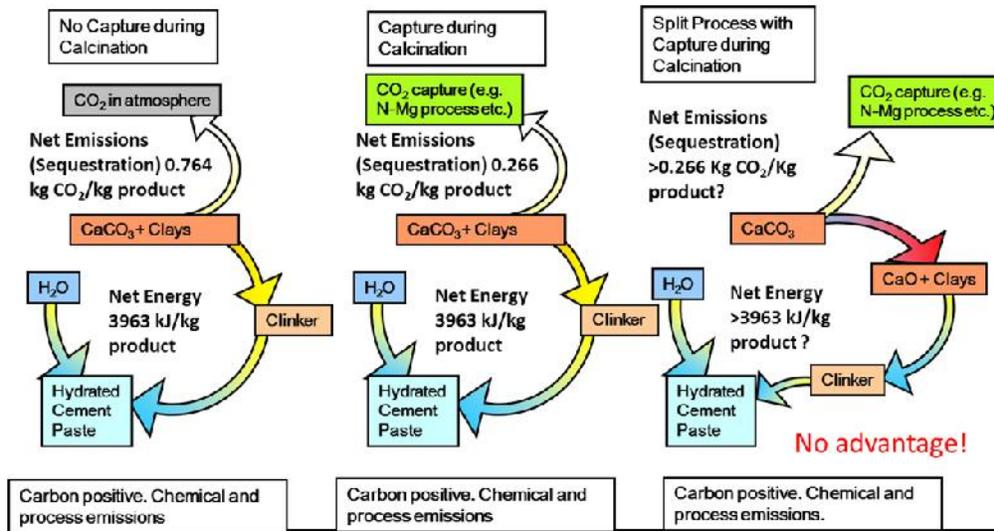
Figure 3 - Options for Portland Cement Manufacture.
