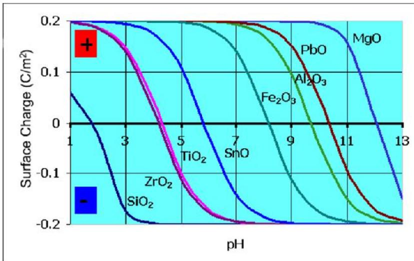
Figure 10 The Change in the Surface Charge of Metal Oxides with pH. (21)
