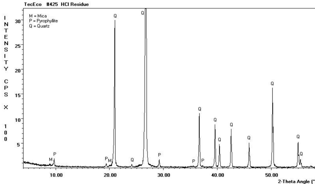
**Figure 2 - XRD Showing Carbonates Before and Minerals Remaining after their Removal with HCl in a Simple Mix (70 Kg PC, 70 Kg MgO, colouring oxide .5Kg, sand unwashed 1105 Kg)**
