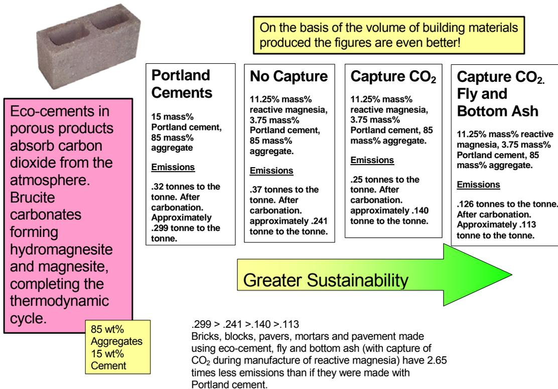
**Figure 3 - The Carbonation of a Typical Eco-Cement Block**
